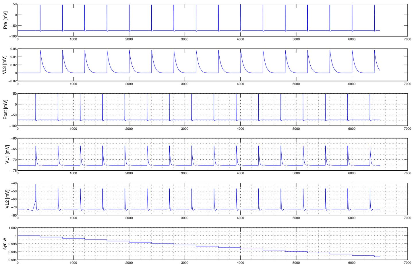
Fig. 2. 16 spike pairs were stimulated at a given timing; this plot shows when it is post-before-pre 80[ms] (which accounts for the observed long-term depression of the synaptic weight,  $w$ ) while the synaptic transmission reliability,  $P$ , is 100% (which accounts for the spiking of the postsynaptic neuron and the updating of the synaptic weight after each presynaptic neural spike). The plot shows various variables of interest that exhibit how the Clopath-Gerstner STDP model works.
